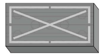
In addition to adhesives, KNAUF Therm ETIXX façade  $\lambda$  31 panels should be fixed with mechanical fasteners with a metal or plastic pin. The minimum number of fasteners should be 4 pcs./m². The places for the installation of mechanical fasteners are marked on the top side of the panel. Proposed anchor installation points are depicted in the pictures below:
